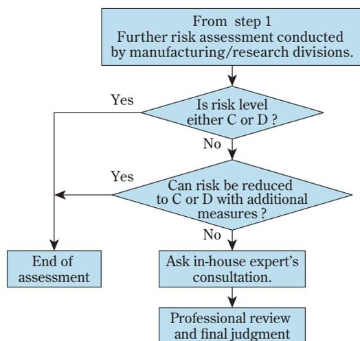
Fig. 2 Flow diagram for electrostatic risk assessment (Step 2)
