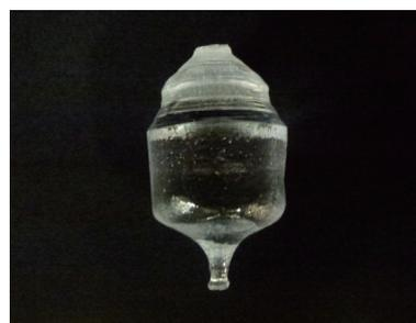
Fig. 13 Image of spinel single crystal
