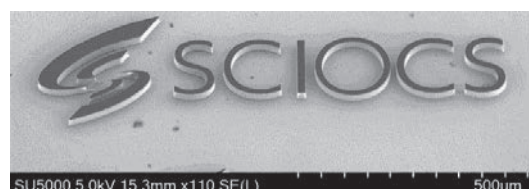
Fig. 12 PEC etched logo pattern of our company “SCIOCS”
