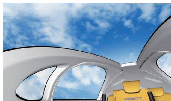
Fig. 1 A cabin space realized by highly stiff and tough transparent resin
