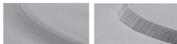
Fig. 14 SEM images of the mesa areas by PEC etching (left) and dry etching (right) 26) Copyright (2019) The Japan Society of Applied Physics
