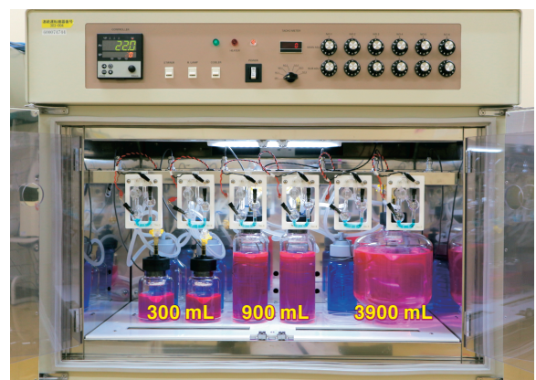
Fig. 4 Coulometer with test vessels that contain 300, 900 and 3900 mL of test media
