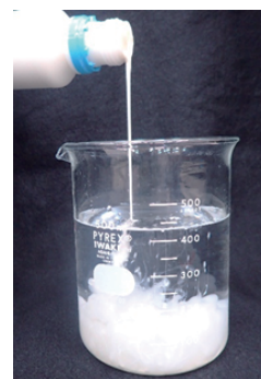
Fig. 15 Dispersion behavior of FUSEKI flowable in water
