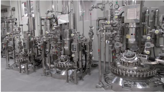
**Fig. 2** Reaction vessels (batch reactors)
