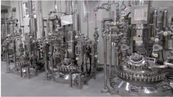
**Fig. 2** Reaction vessels (batch reactors)
