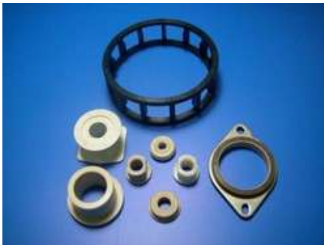
Figure 6-5-1 Photograph of a Molding of SUMIPLOY
